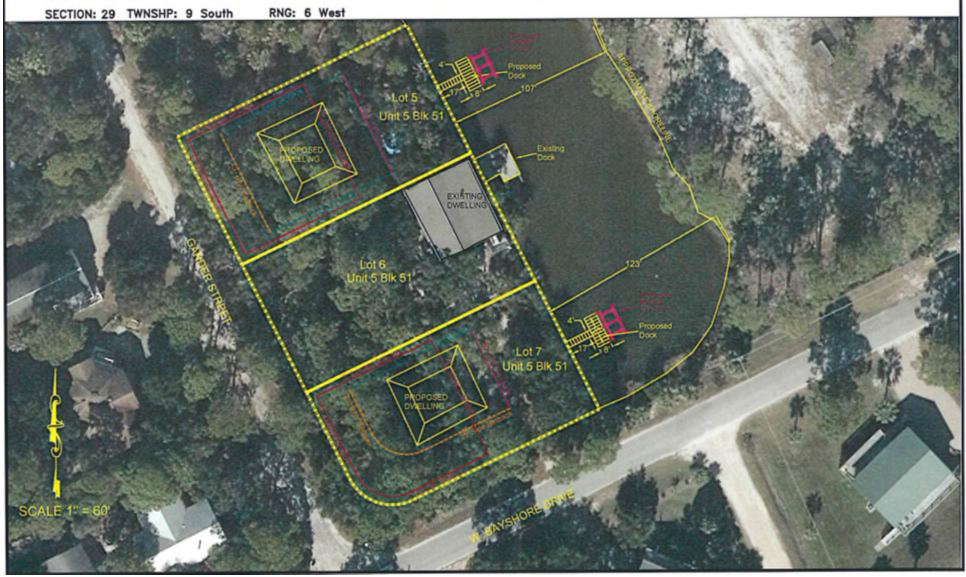
3- **RECOMMENDED APPROVAL:** (Unanimous) Consideration of a request to construct a Single Family Dock located at Lot 5, Block 51, Unit 5, 305 Gander Street, St. George Island, Franklin County, FL. The proposed access walkway for the dock will be constructed 17' x 4' with a terminus 8' x 20'. One 10' x 20' boat lift. Total square footage of the dock will be 428 sq ft. Request submitted by Dan Garlick, Garlick Environmental Associates Inc., Agent for Rudy Rowe, applicant. (Proposed future house.)
