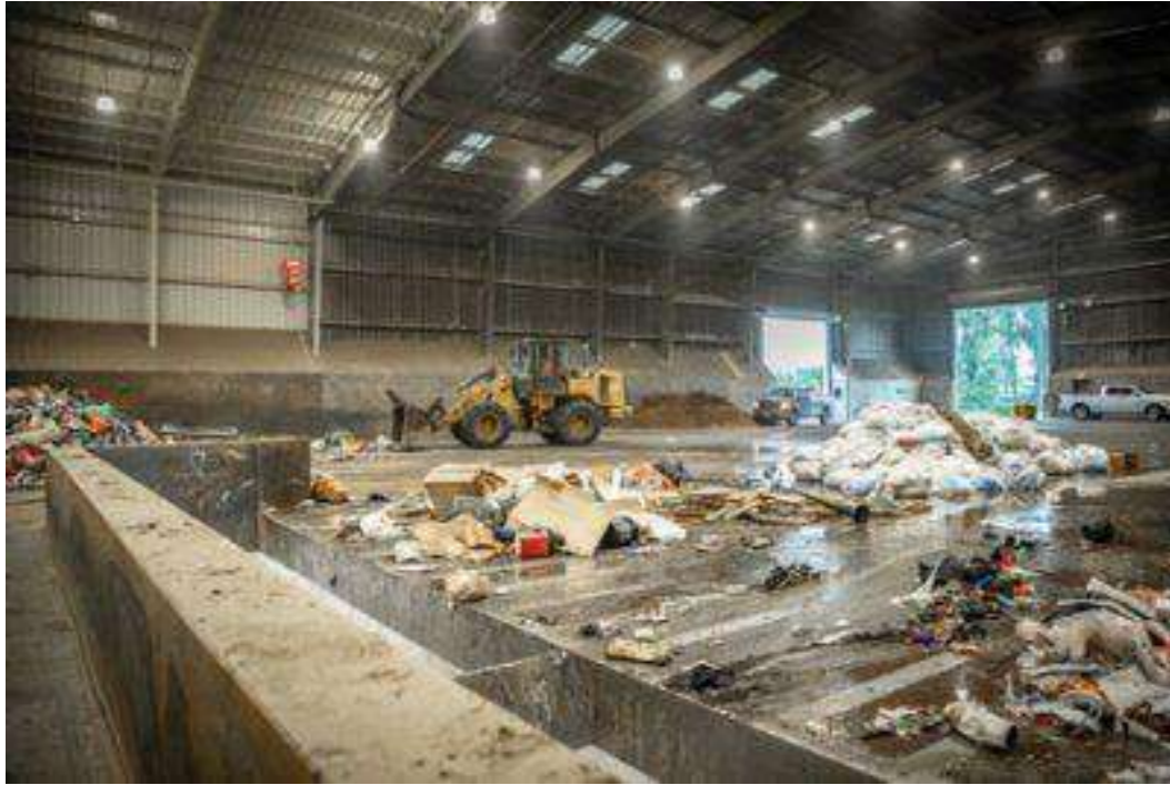
Figure 1 – MSW Transfer Station Tipping Floor, Hopper, and Wheel Loader
